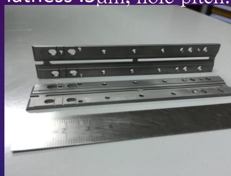
Thine plate processing Flatness :5 \mu m, hole pitch:5 \mu m
